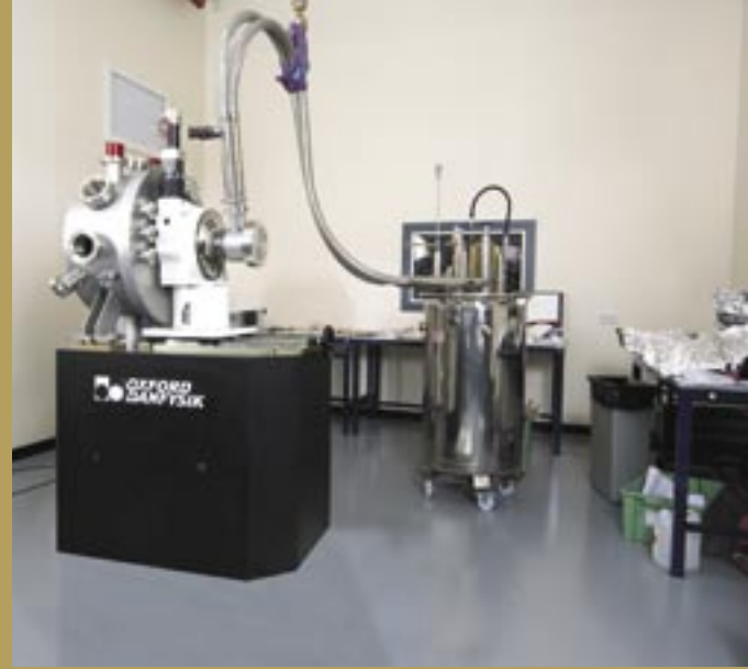
One of the DCMs for the DLS fully assembled in the cleanroom in Oxford
