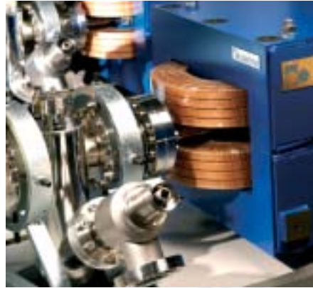
Vacuum chamber and magnet details on the CLS 2.9GeV Booster Synchrotron
