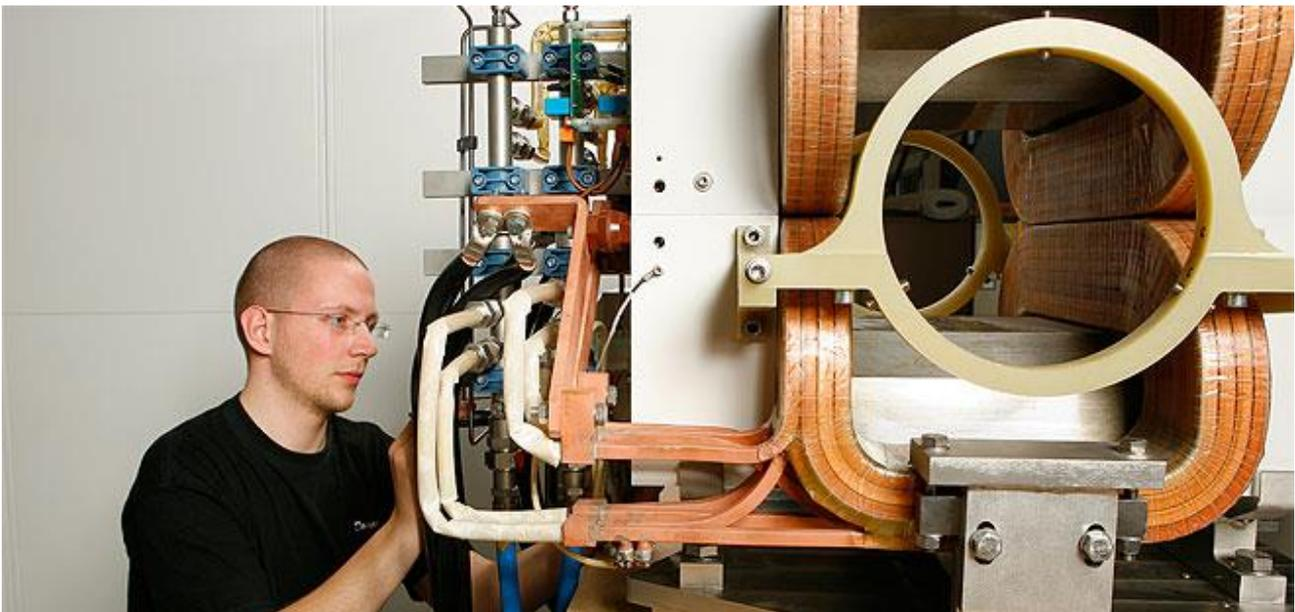
*10Hz Slow Kicker Magnets with Pulsed Power Converters for ISIS 2nd Target Station at Rutherford, UK*
